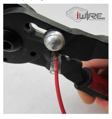
6. Pull test the crimp. It should stay in place even with moderate pulling. Be careful not to pull too hard because it will stress the joint.
